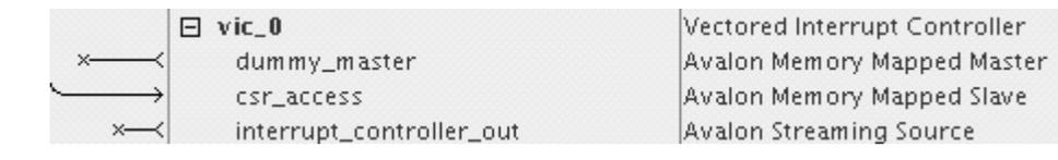
After adding a VIC to the SOPC Builder system, you must parameterize the VIC and the EIC interface at the system level. Immediately after you add the VIC, several error messages appear. Resolve these error messages by executing the following actions in any order:
