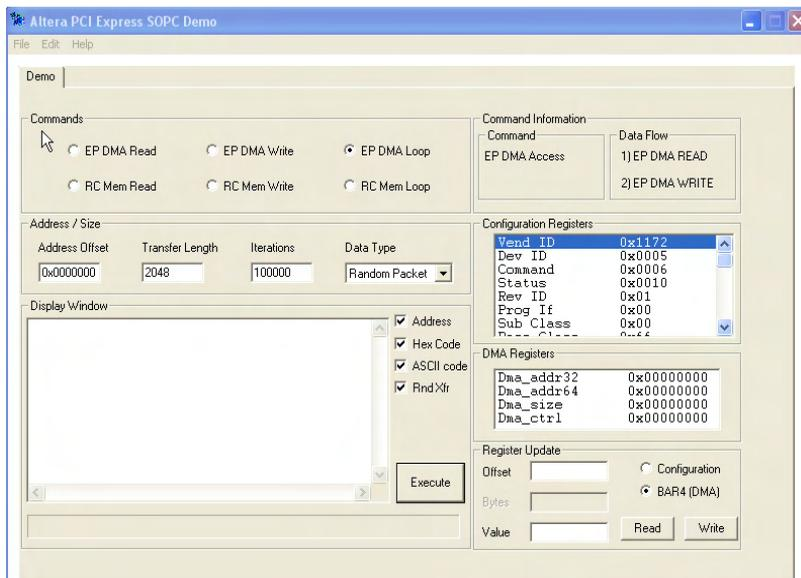
By default, the Demo interface is set up to run a DMA loopback test. You can run this test by clicking the **Execute** button. You can also use this interface to perform tests that include memory read and write transactions or to read the configuration registers.
