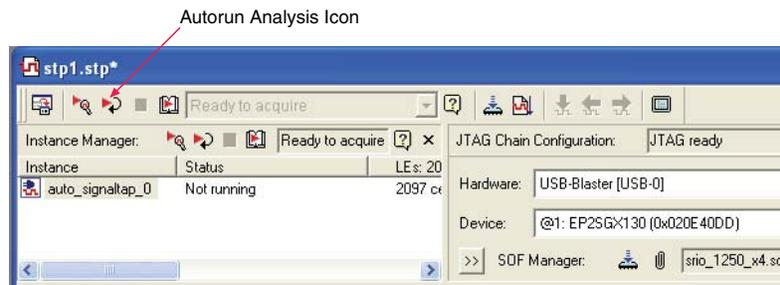
Figure 18 shows the SignalTap II Embedded Logic Analyzer. The window displays activity on the I/O slave write interface of the RapidIO MegaCore function.
