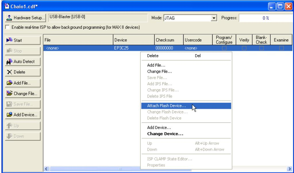
Figure 15. Selecting Flash Device
