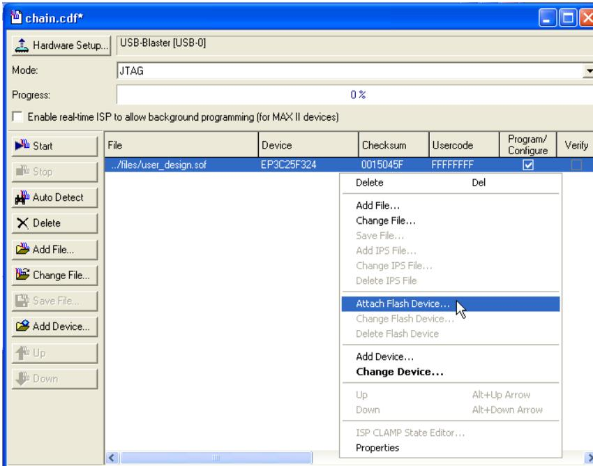
Figure 21. Selecting Flash Device
