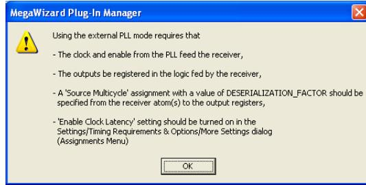
This warning dialog box displays a list of requirements necessary to take advantage of the Stratix II fast PLL features. Selecting not to register the outputs of the receiver requires the following:
