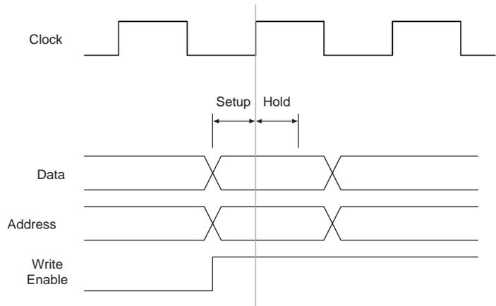
In many designs, even if the memory is asynchronous, the modules the memory interfaces with are synchronous, making the conversion to synchronous memory design straightforward. Registers in the data path would move into the memory block, having a negligible effect on functionality.
