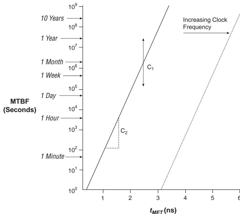
The constant  $C_1$  scales the MTBF equation linearly, shifting the entire curve up or down. The constant  $C_2$  affects the slope of the MTBF vs.  $t_{MET}$  curve. Increasing the clock frequency shifts the entire curve to the right, lowering the MTBF value for a given settling time.
