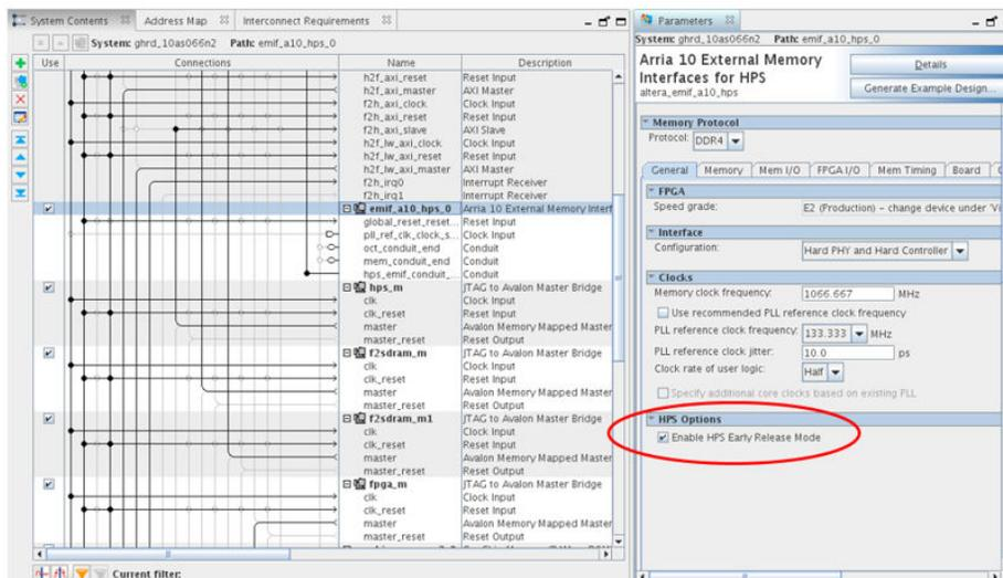
Selecting this option parameter in the Intel Arria 10 HPS EMIF disables the component reset signal from the FPGA core logic. Setting this option is important to ensure that the EMIF does not accidentally reset when loading the FPGA core image.
