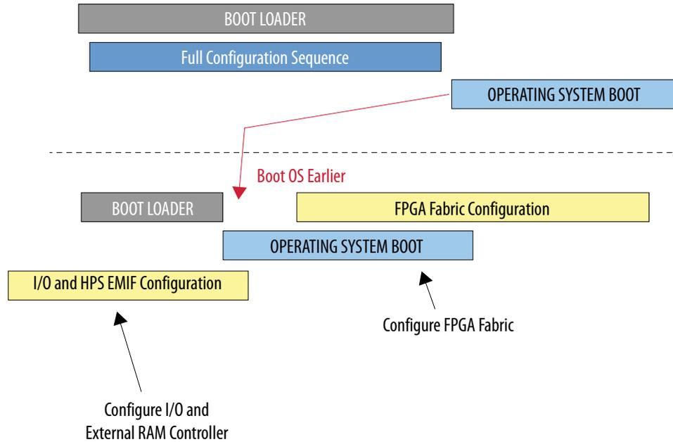
Some designers might want to boot the HPS operating system (OS) immediately. This action can be accomplished by postponing FPGA fabric configuration until the OS has booted. Booting the OS quickly is achieved by using the boot loader to only configure the FPGA I/O, Shared I/O and external memory before FPGA fabric is configured, then allowing the OS to boot and configure the FPGA fabric.
