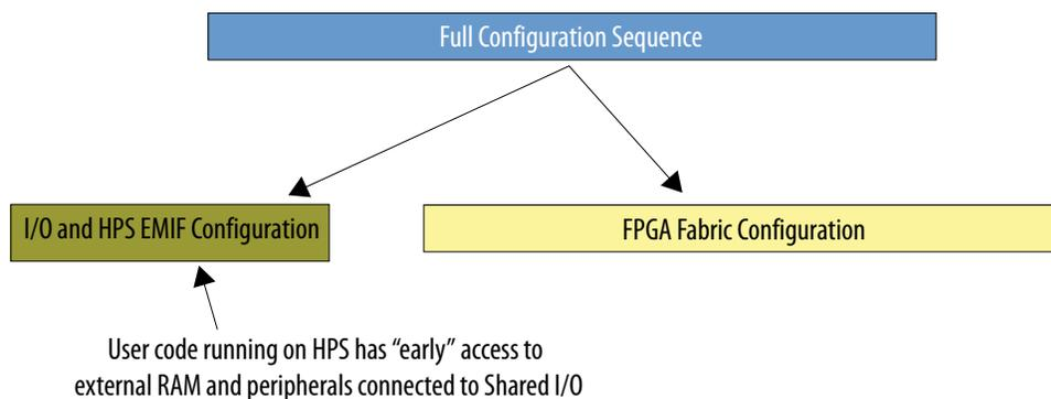
Splitting the configuration sequence provides HPS access to Shared I/O and EMIF before the FPGA fabric is configured. This allows more flexibility for designs that need faster boot times or alternate boot sources.
