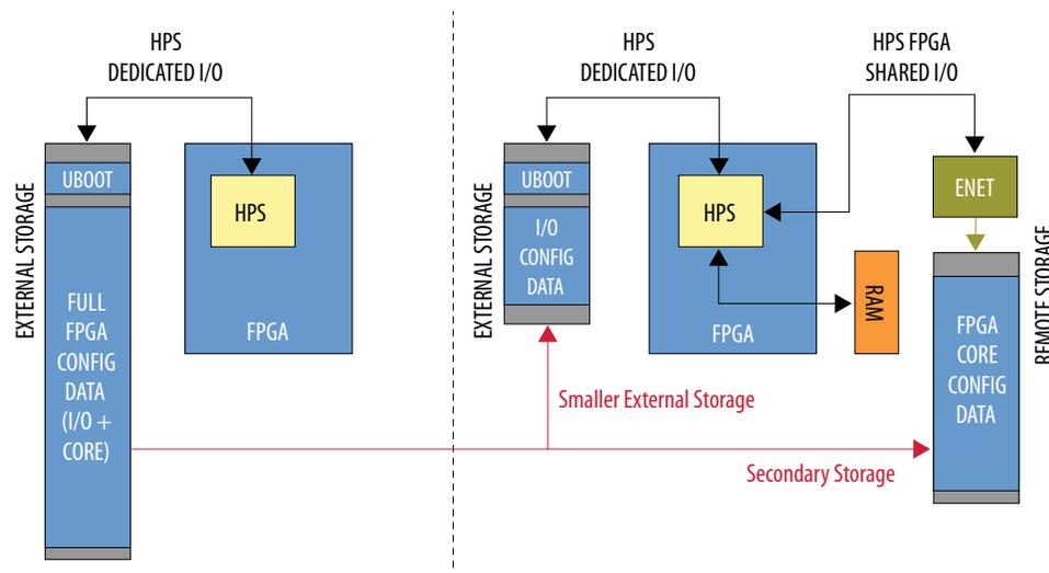
Another reason to enable the Early I/O Release feature is to gain boot software access to an interface connected to Shared I/O, such as a secondary mass storage device or network connection. This secondary access allows the primary storage connected to the HPS dedicated I/O pins to be smaller and possibly even write protected.
