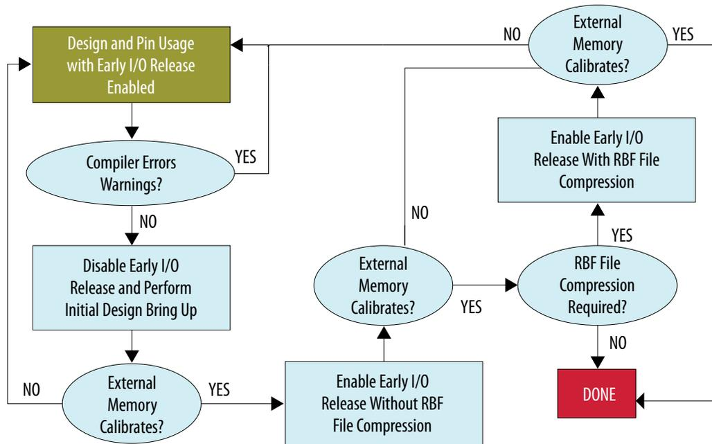
After you confirm that configuration and external memory calibration is successful with Early I/O release disabled, Intel recommends you enable the Early I/O Release without **.rbf** file compression. Testing the Early I/O Release feature without **.rbf** file compression helps determine that your design is properly implementing the flow as described in this document.
