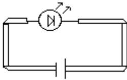
2. One at a time, bend foil strips into the pattern matching the design you have on your cardboard. Lay the foil strips directly onto the pattern and tape them into place. Be careful not to place the tape close to the ends of the strips because the ends are needed as connection points.
