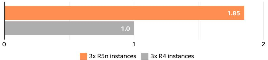
Figure 1. Relative test results comparing the Weathervane 2.0 performance of the small (eight-vCPU) R5n instance type to the small R4 instance type.
