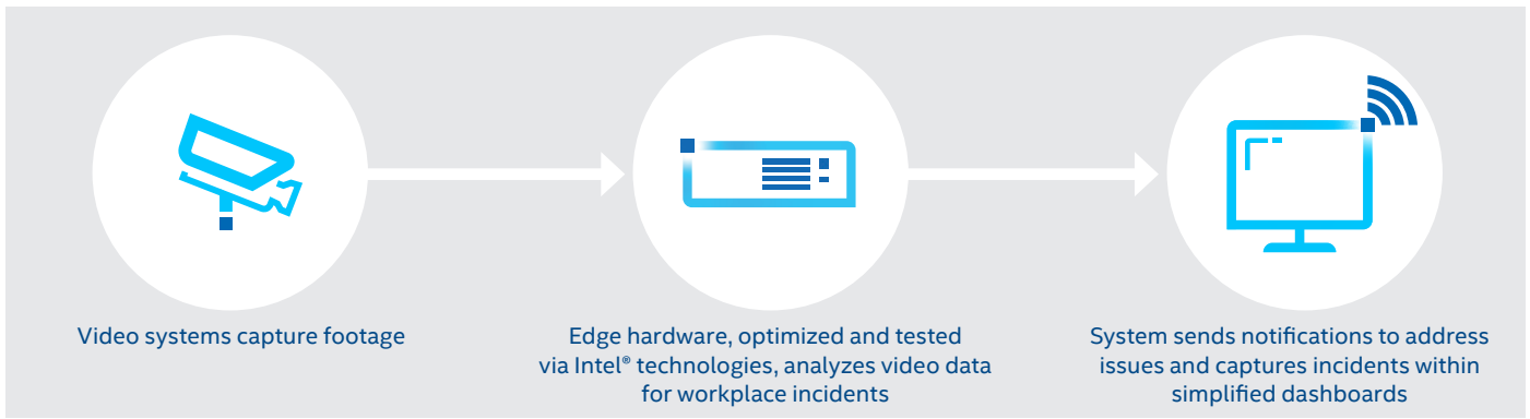
Figure 1. The Vulcan AI WorkSafe solution uses video data from workspace cameras and CCTV systems to identify safety hazards. Integrated notification, alerting, and logging features disseminate the right information to the right people as issues occur, empowering them to quickly take action to remediate the issue.
