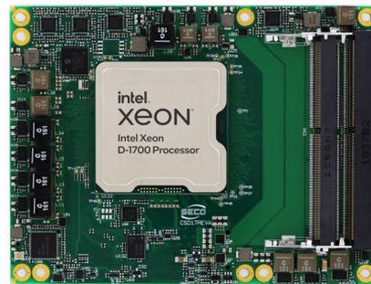
Figure 1: The SECO JULIET COM Express® Basic Type 7 module with Intel® Xeon® D-1700 processor.
