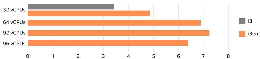
Figure 2. Relative DVD Store 3 scale-up test results comparing total performance (in orders per minute) achieved by three-host software-defined data center using AWS i3 and i3en instances with VMs at increasing vCPU counts. Higher is better.
