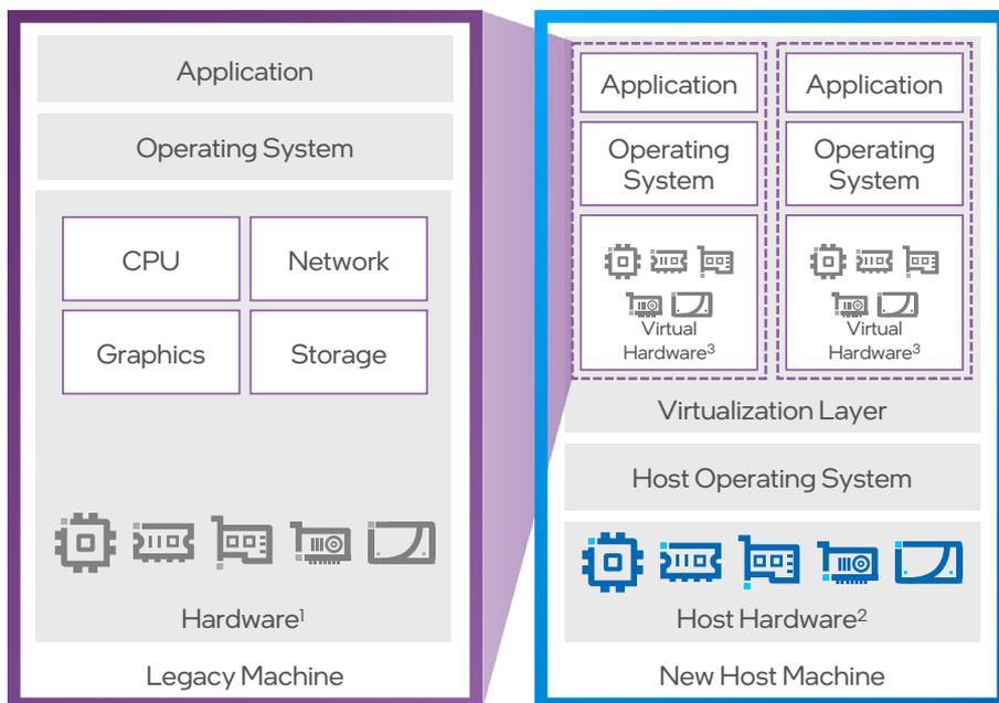
**Figure 3.** The legacy solution compared to the new virtualization solution. When Intel migrated to the new environment, a virtualization layer was added on top of the OS. The added layer allowed Intel to virtualize legacy content in the host machine.
