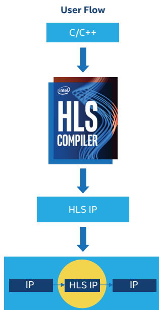
Figure 1. Intel HLS Compiler Tool Flow
