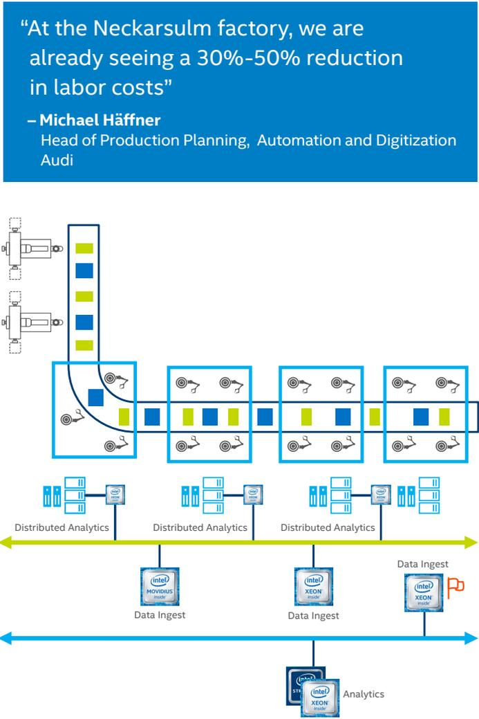
**Figure 1.** Audi's solution ingests data from the welding-gun controllers and analyzes it at the edge. A machine-learning algorithm was trained to detect faulty welds. Audi's solution ran an Intel® Xeon® processor but it can scale from Intel® Core™ processors all the way to Intel® Xeon® processor E and Intel® Xeon® SP server processors with no changes to the software.
