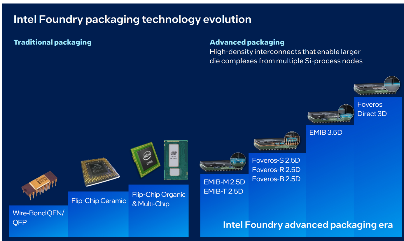
Figure 3. Evolution of Intel packaging technology, from traditional to advanced packaging.
