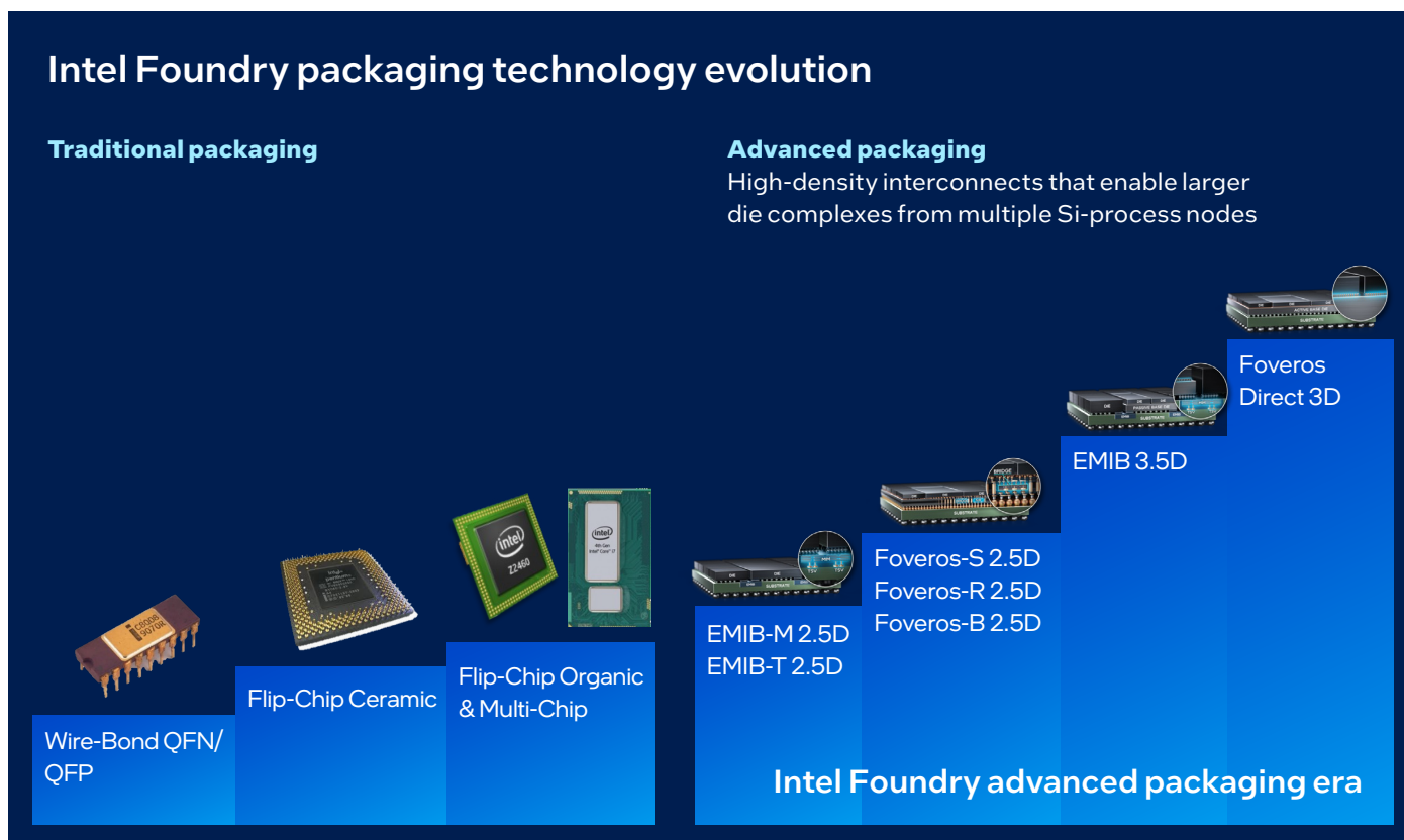
Figure 3. The Intel packaging technology revolution, from traditional to advanced packaging.
