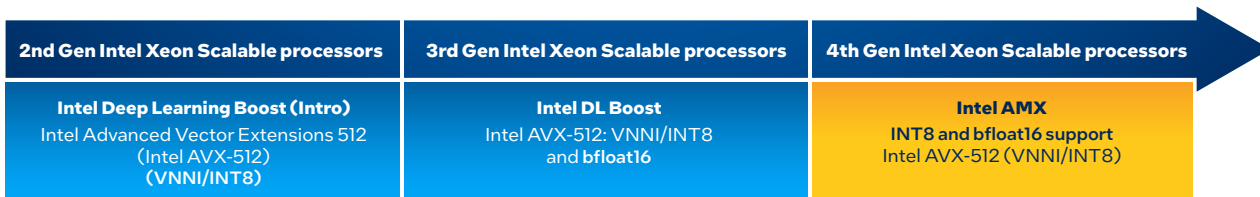
Figure 3. Innovations like Intel AMX build on the accelerators built into previous-generation Intel Xeon Scalable processors, enabling even greater performance
