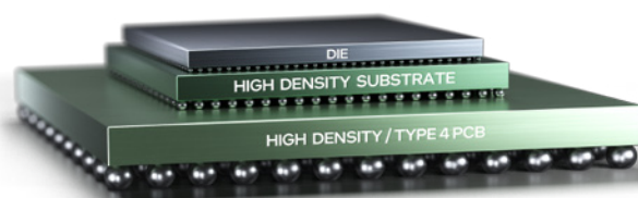
Figure 6. A high density “patch” with finer features is sandwiched between an active chip (top) and a PCB-like interposer (bottom).
