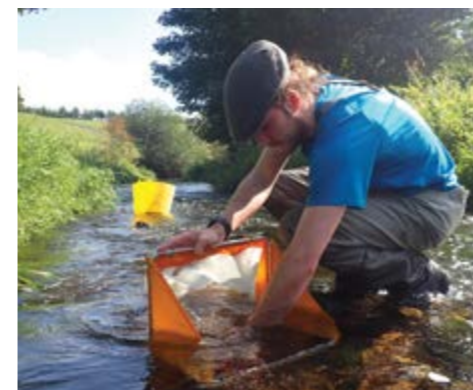
A Surber sampler is used to measure the number of crayfish per unit area
