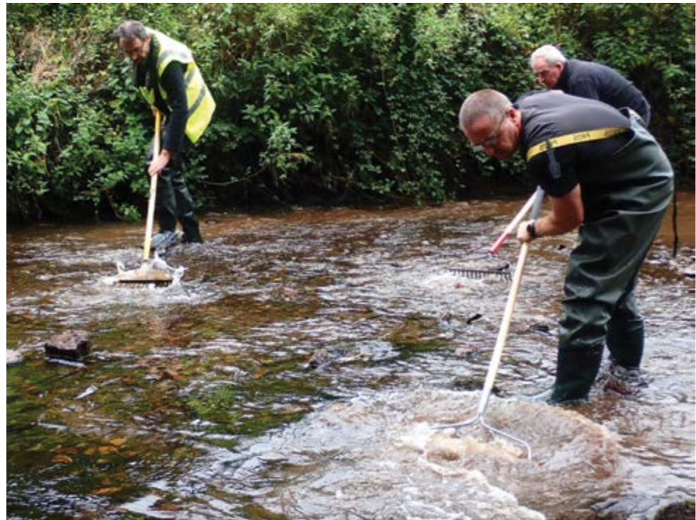
A modified Surber sampler was used to quantify the presence of certain particle sizes on the riverbed
