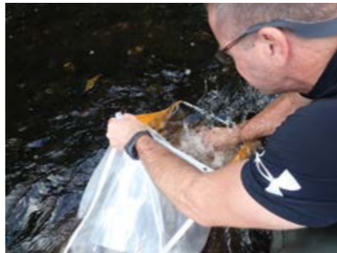
A modified Surber sampler was used to quantify the presence of certain particle sizes on the riverbed
