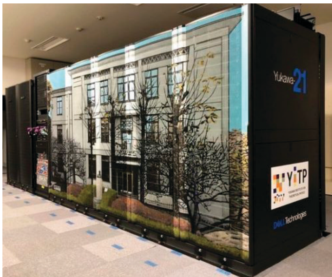
The Yukawa-21 system features Dell EMC PowerEdge R840 platforms with 28-core Intel Xeon Platinum 8280 processors. (Photo courtesy YITP)
