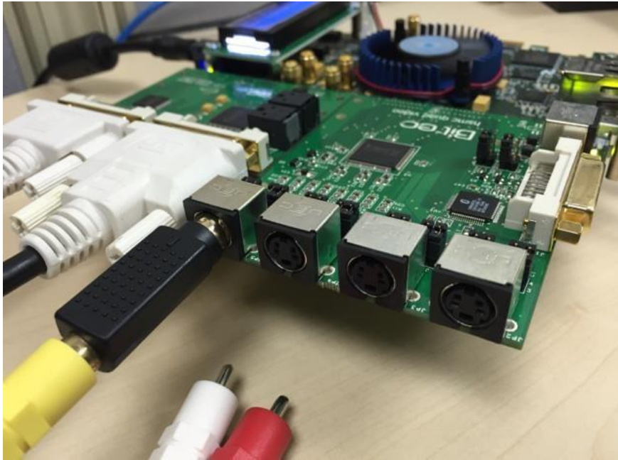
Figure 12 - Composite Video Connection to Quad Video Daughter Card
