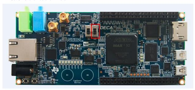
The logic within the FPGA can be reset by sliding the switch (SW0) up. To release reset, slide SW0 back down to the default position
