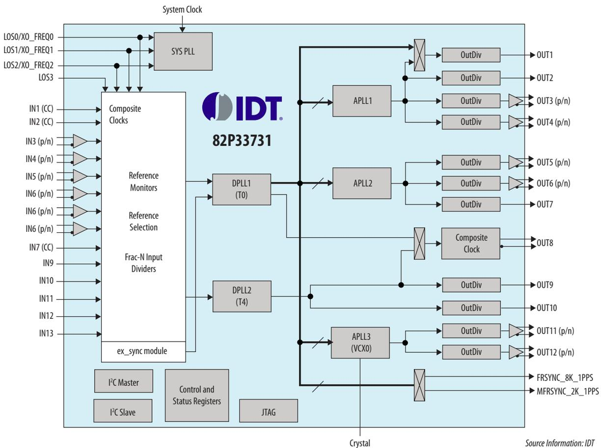
As shown in Figure 2, the SETS has multiple clock inputs, both single-ended and differential, that can be driven by recovered clocks from the Altera FPGA. The SETS uses DPLL1 to clean a selected recovered clock. DPLL1 meets the frequency accuracy, pull-in, hold-in, pull-out, noise generation, noise tolerance, transient response, and holdover performance requirements of ITU-T G.8262.
