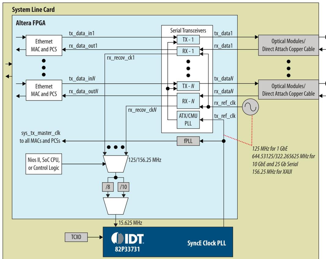
Figure 2. 82P33731 Synchronous Equipment Timing Source
