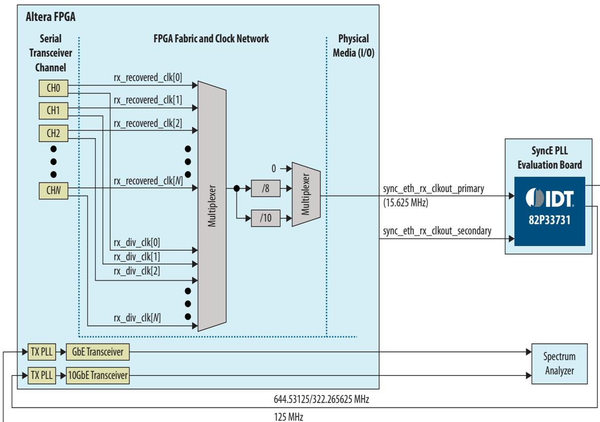
The FPGA implemented 16 Ethernet 10GBASE-R channels using the Altera 1G/10Gb Ethernet MAC core with the Altera 10GBASE-R PHY IP core. Because the Ethernet cores are small, a Gray-code noise generation core was added to the design so that 71% of the FPGA resources were used, mimicking the switching noise that might be present in a line card with additional application logic.
