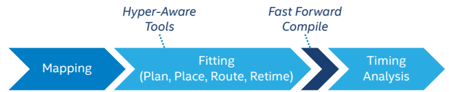
Figure 2. Intel HyperFlex FPGA Architecture Design Flow
