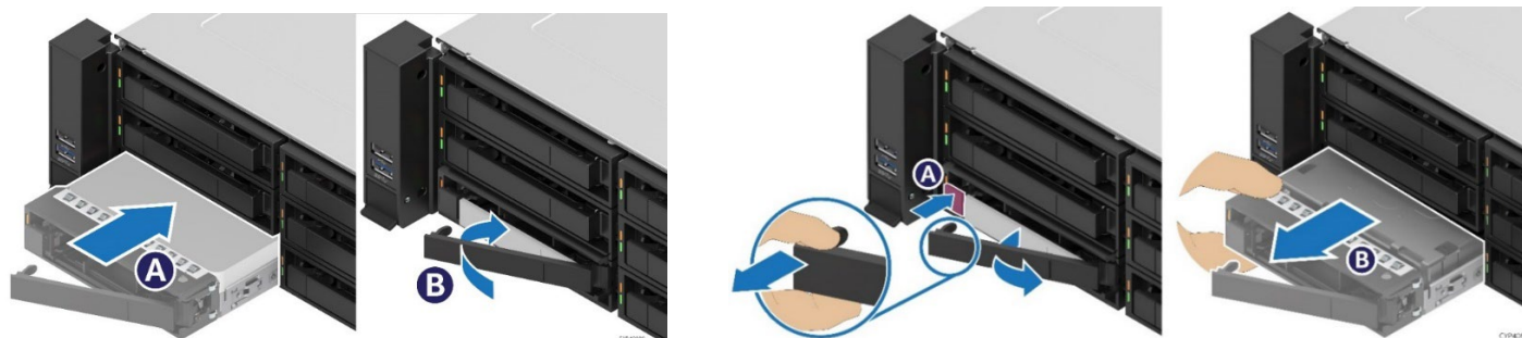
Figure 64. 3.5" Drive Insertion / Extraction
