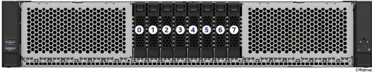
Figure 70. 8 x 2.5" Front Bay Drive Configuration – M50FCP2UR208
