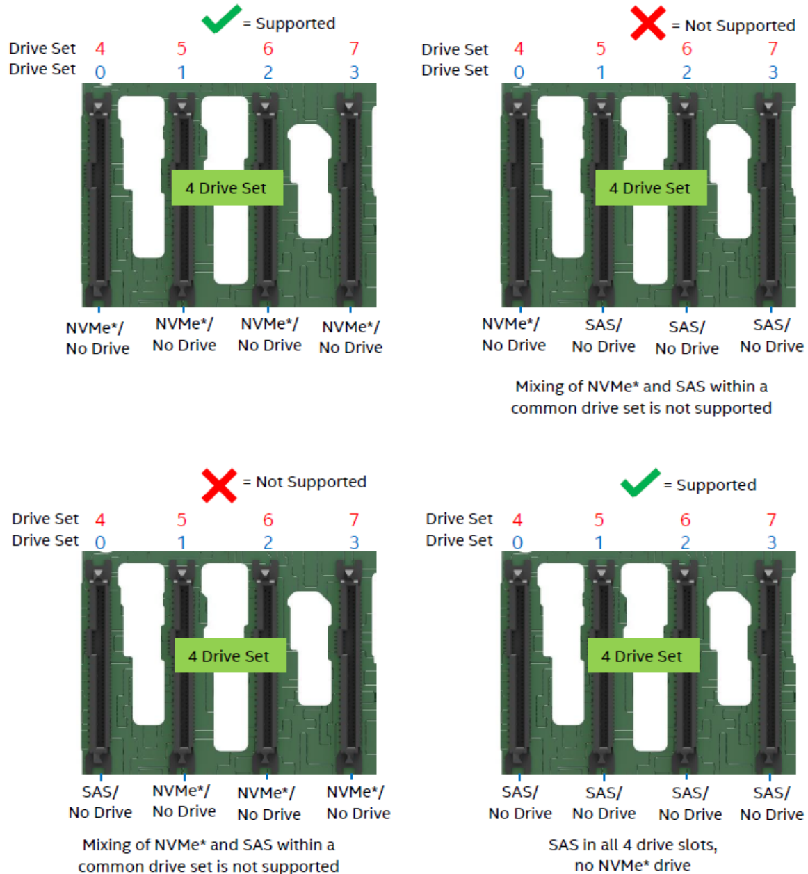
Figure 86. Supported Drive Population for Server Board MCIO Connectors or Tri-Mode Intel® RAID Module
