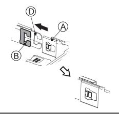
(2) Install the outer member Install  $\bigcirc$  onto  $\bigcirc$  .
