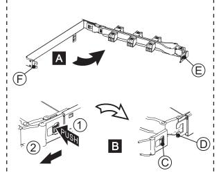
(3) Release the inner member Press the "PUSH" button on the CMA plug-in part to draw
