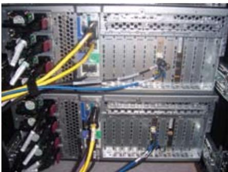
**Figure 2.** Configuration of the server wiring when two 10G connections replace eight 1GbE connections.
