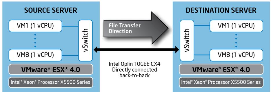
Figure 12. Test configuration for Case 3.
