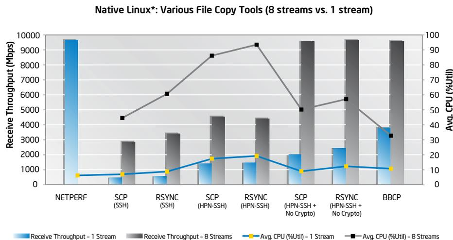
Figure 6. Comparison of various file copy tools (eight streams).
