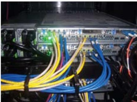
**Figure 1.** Configuration of the server wiring when using eight 1GbE connections.
