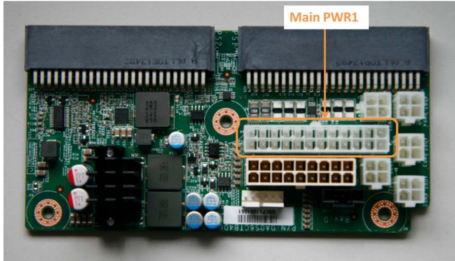
Figure 2. Location of the 2x12 pin connector (labeled "Main PWR1") on the PDB
