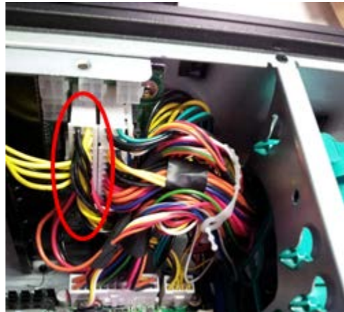
Figure 6. Location of the "Main PWR1" connector
