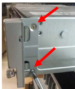
Figure 3. Front Panel Assembly Attach Points
