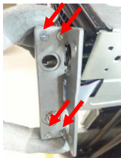
Figure 4. Front Panel Housing Attach Points
