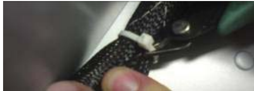
Figure 11. Removing the Cable Tie (Close-Up)
