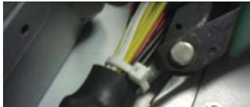
Figure 10. Removing the Cable Tie
