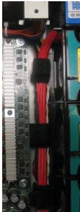
Figure 26. Velcro* Tie Wraps Tucked Into Place
