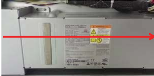
Figure 6. Sliding the Cage to Release the Locking System
