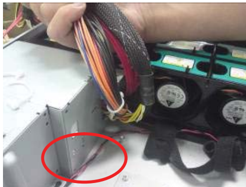
Figure 12. Cable Not Removed From Bundle
