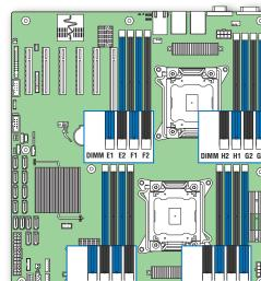
Memory Type: Minimum of one 1 GB, DDR3 800/1066/1333/1600 MHz UDIMM/RDIMM/LRDIMM.
