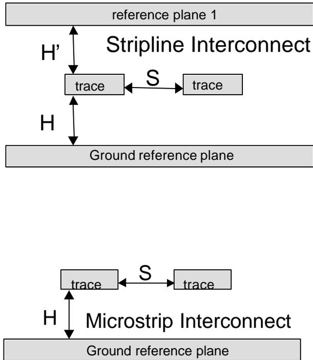
Figure 3-12: Spacing to Height Definitions for Stripline and Microstrip Implementations
