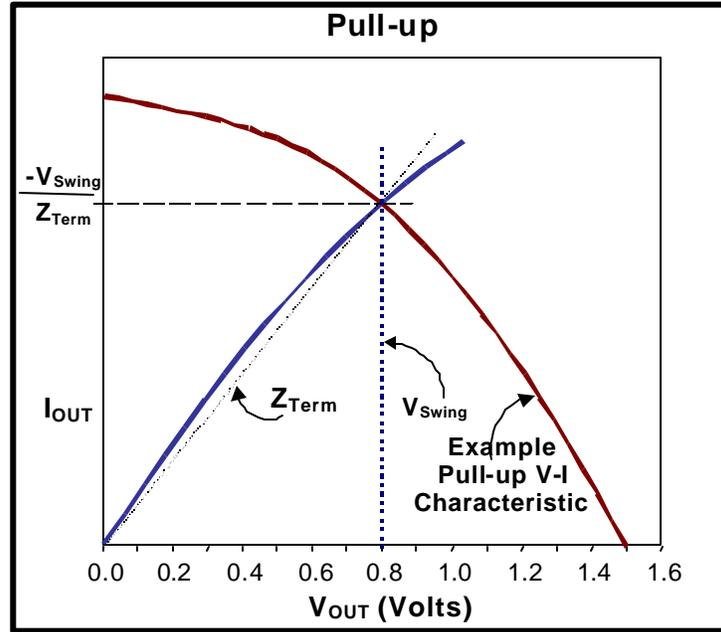
Figure 3-22: V/I Curve for AGP3.0 Transmitter Pull-up
