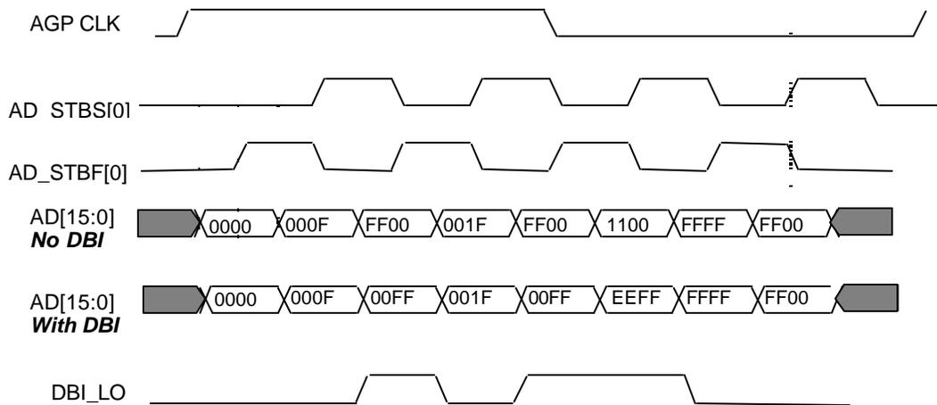
Figure 2-7: Usage of DBI on Source Synchronous Transfers
