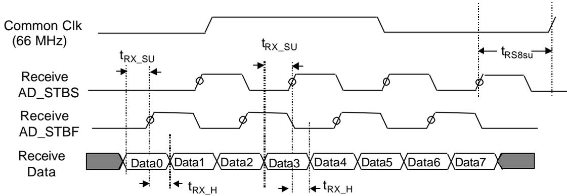
Figure 3-5: Receive Strobe/Data Timings for 8X Source Synchronous Timing
