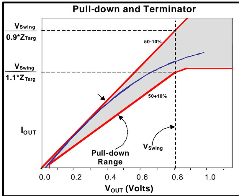
Figure 3-21: V/I Curve for AGP3.0 Receiver Termination Device
