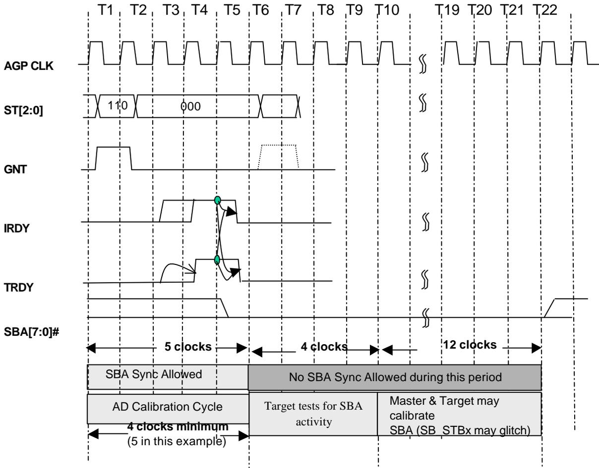
Figure 2-6: SBA Calibration When SBA Strobes are Stopped
