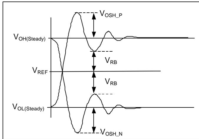
Figure 3-16: General Signal Integrity Waveform
