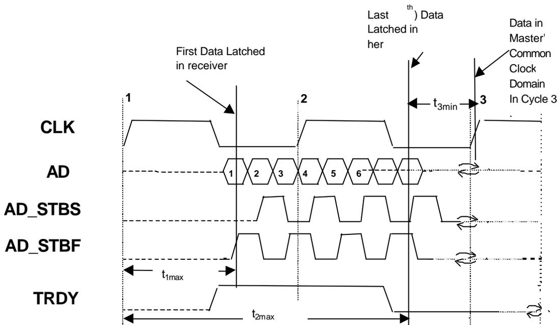
Figure 2-2: 8X Data Transfers on AD Interface
