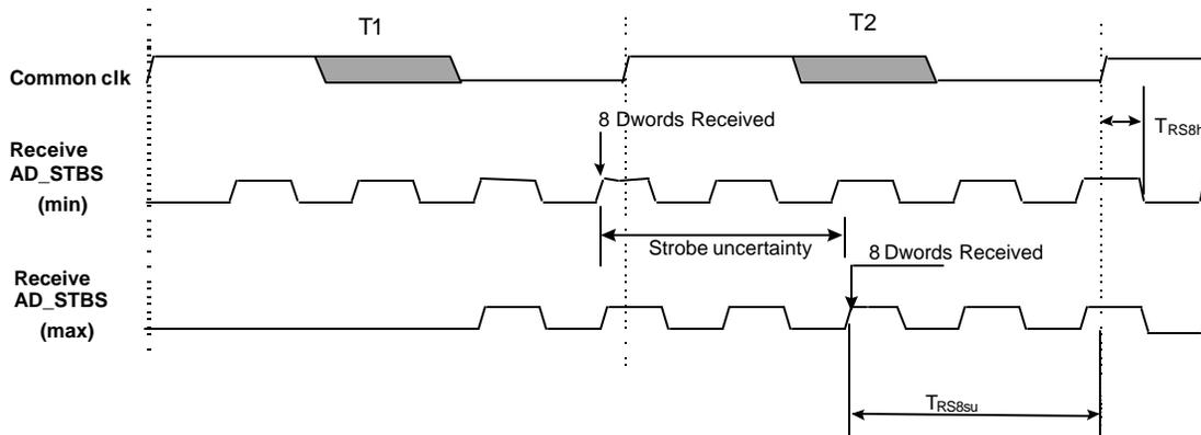
Figure 3-6: Minimum and Maximum Inner to Outer Loop Receive Timings
