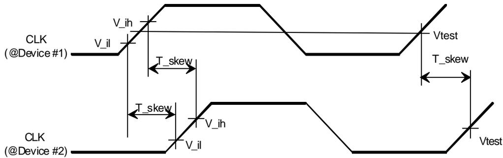
Figure 3-13: Clock Skew Diagram
