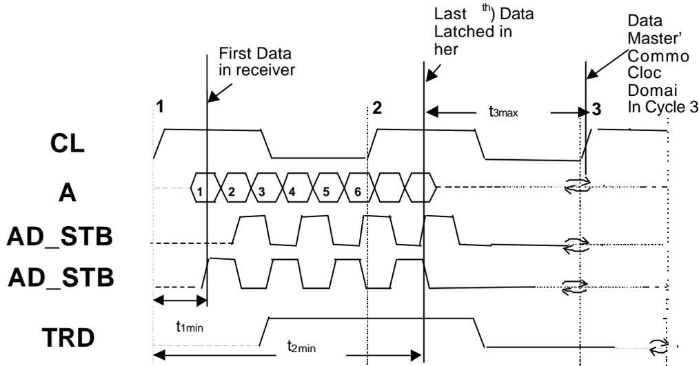
Figure 2-3: Minimum TRDY and AD\_STB Timing Relationship
