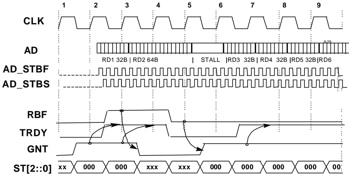
Figure 2-9: Use of RBF in Read Transaction Control
