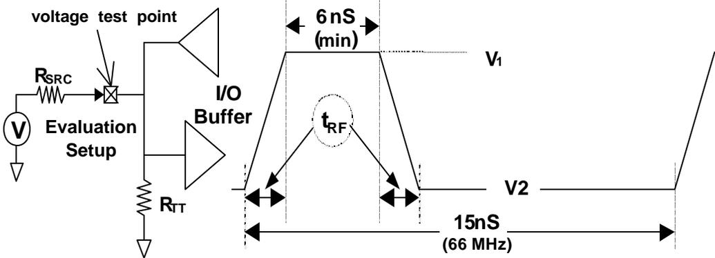
Figure 3-20: Open-circuit Voltage
