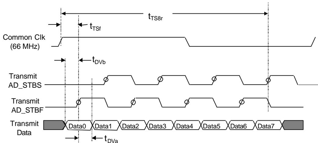
Figure 3-4: Transmit Strobe/Data Timing for 8X Source Synchronous Timing
