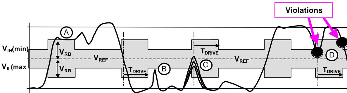
Figure 3-19: Address/Data Ringback Examples
