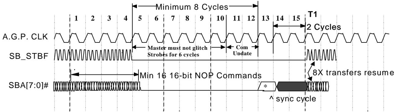
\* Since SBA has inverted polarity in AGP3.0, the logical value of Sync = FEh while the electrical value is LLLL LLLH.
