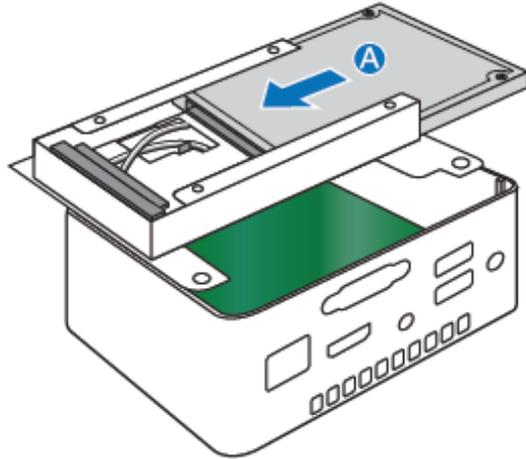
3. Secure the drive into the drive bay with the two small silver screws that were included in the box.
