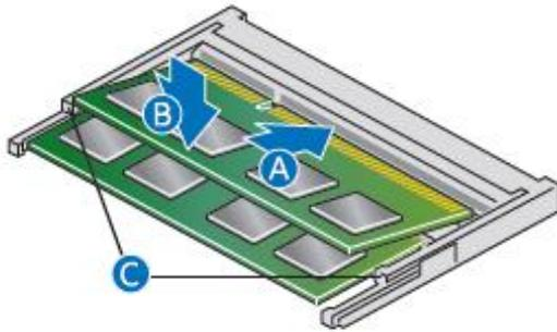
3. Align the small notch at the bottom edge of the SO-DIMM with the key in the socket.
