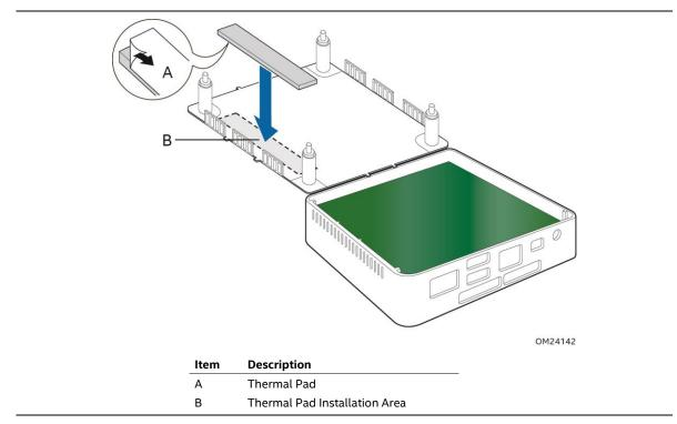
Figure 19. Installation Area of Thermal Pad for Intel NUC Kit NUC5i5RYK/NUC5i3RYK
