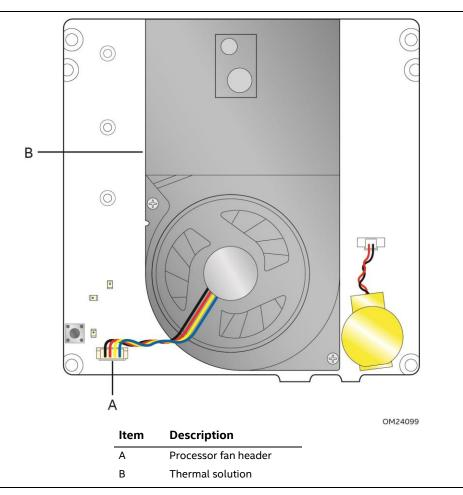
Figure 7. Thermal Solution and Fan Header
