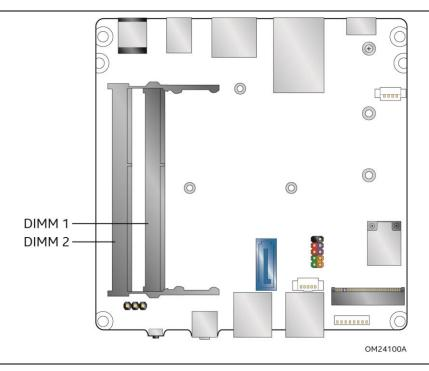
Figure 4 illustrates the memory channel and SO-DIMM configuration.
