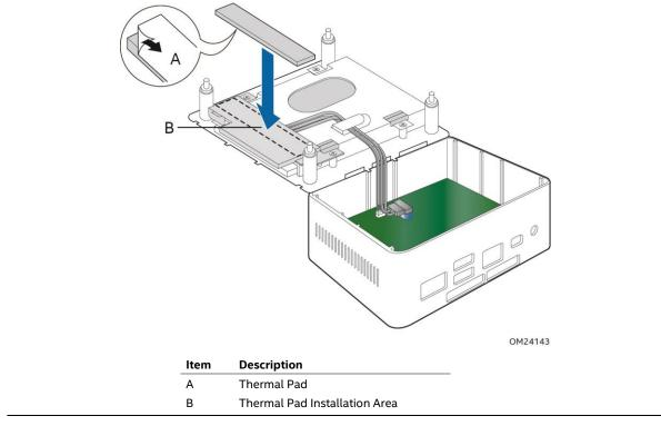
Figure 20 shows the installation area of the thermal pad for the Intel NUC Kit NUC5i5RYKH/NUC5i3RYKH.
