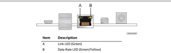
Figure 6. LAN Connector LED Locations
