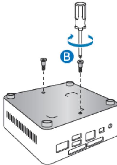
2. Attach the two slightly larger black screws to the bottom chassis cover of the Intel NUC.
