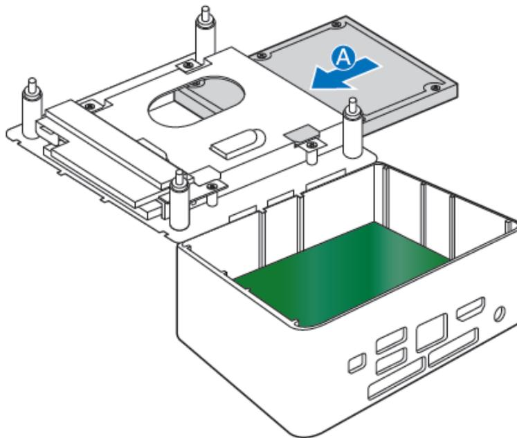
2. Secure the drive into the drive bay with the two small silver screws that were included in the box.
