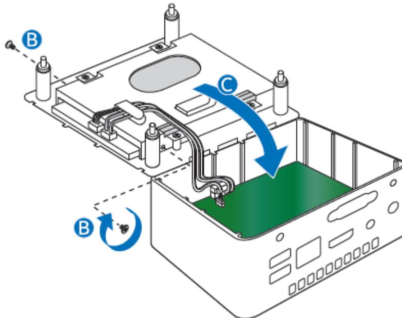
4. Set the drive bay bracket down inside the chassis (C), taking care not to pinch the SATA cables along
