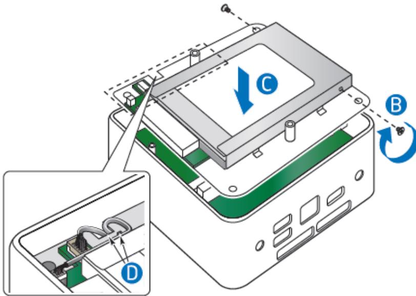
4. Set the drive bay bracket down inside the chassis (C), taking care not to pinch the SATA cables along the edge (D).
