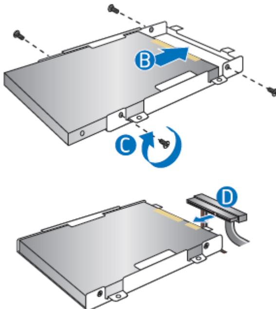
4. Set the drive bay bracket down inside the chassis, taking care not to pinch the SATA cables along the edge. Secure the drive bay with the screws.
