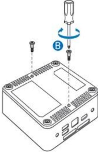
2. Attach the two slightly larger black screws to the bottom chassis cover of the Intel NUC.
