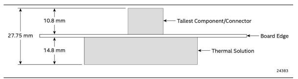
Figure 17. Board Height Dimensions
