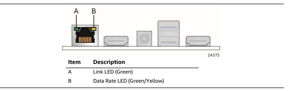
Figure 5. LAN Connector LED Locations
