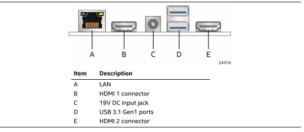
Figure 10. Back Panel Connectors
