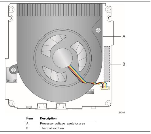
Figure 18. Localized High Temperature Zones
