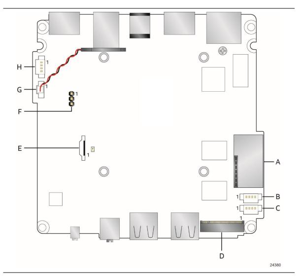
Figure 12. Connectors and Headers (Bottom)
