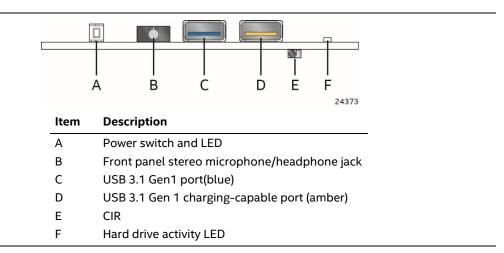
Figure 9. Front Panel Connectors, Controls and Indicators
