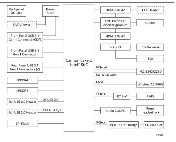
Figure 3. Block Diagram
