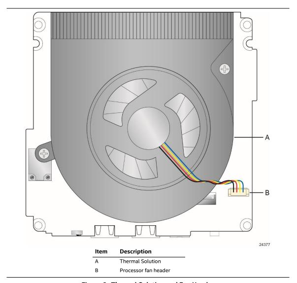
Figure 6. Thermal Solution and Fan Header
