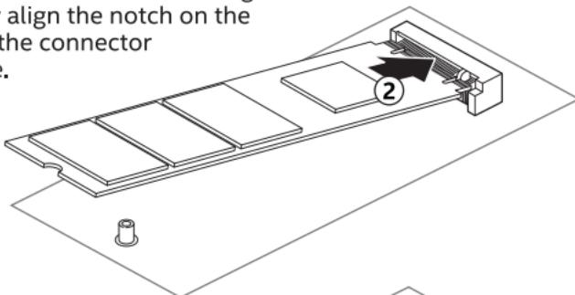
Push the M.2 card down and re-install screw into standoff to secure.
