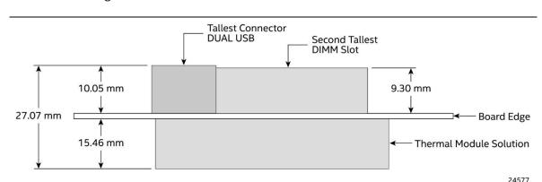
Figure 16 shows the height dimensions of the board. Dimensions are in mm.
