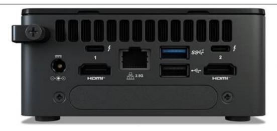
Figure 13. Tall Chassis Image Back Panel
