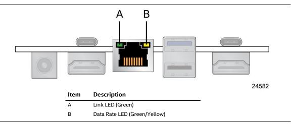
Figure 7. LAN Connector LED Locations
