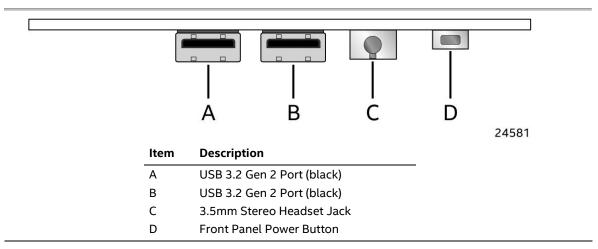
Figure 3. Front Panel Connectors
