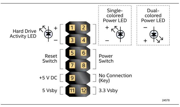
Figure 8. Connection Diagram for Front Panel Header (2.0 mm Pitch)
