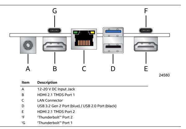
Figure 4. Back Panel Connectors
