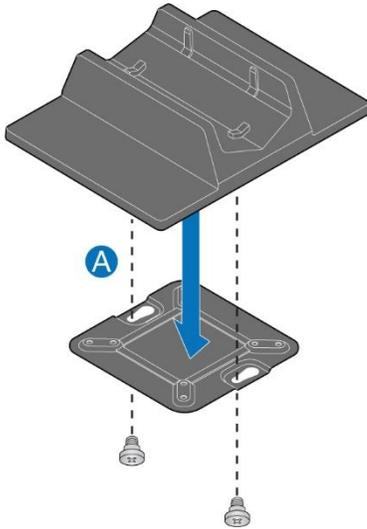
2. Using the four small black screws that were included in the box, attach the VESA bracket to the back of the monitor or TV
