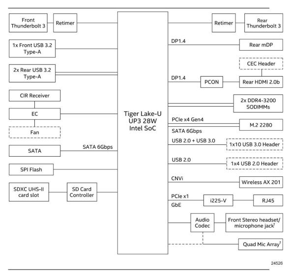
Figure 5. Block Diagram
