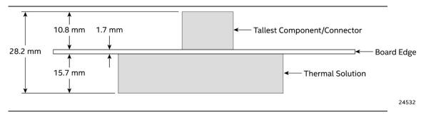
Figure 10. Board Height Dimensions
