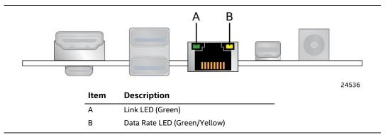
Figure 7. LAN Connector LED Locations
