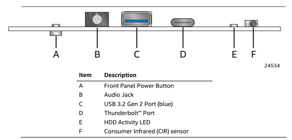
Figure 3. Front Panel Connectors
