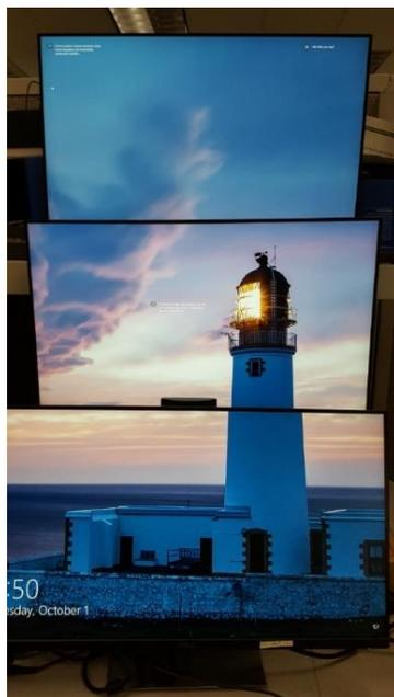
**Figure 8: Vertical Combined Desktop Display Mode – 3 enabled**
