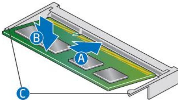
3. Align the small notch at the bottom edge of the SO-DIMM with the key in the socket.
