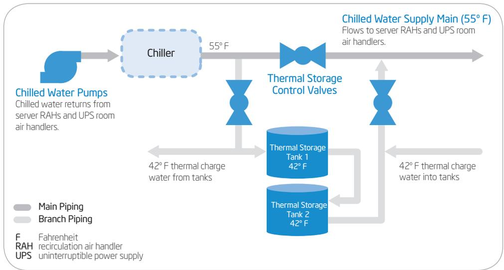
**Figure 2. Diagram of supplemental thermal storage system loop.** The valve on the main chilled water supply line is open during normal operation. In the event of an outage, this valve closes and the two valves on the thermal storage branch piping open to allow the water in the storage tanks to flow into the chilled water supply, providing cooling to the air handlers.
