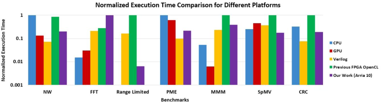
**5** Performance of our work compared to existing CPU, GPU, Verilog\*, and FPGA OpenCL implementations. Our work outperforms CPU and OpenCL for most of the benchmarks. Moreover, we also achieve speedups over GPU (SpMV, PME) and Verilog (SpMV, Range Limited).
