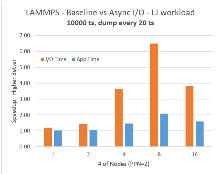
**1 Speedup from MPI I/O time and total run time for LAMMPS**
