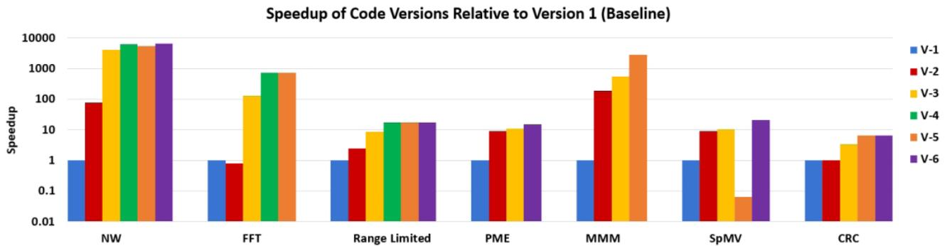
**2** Impact of systematic application of the proposed optimizations to a cache-optimized CPU baseline code. In almost all cases, every subsequent code version shows increasing performance, with up to orders of magnitude better performance possible for fully-optimized
