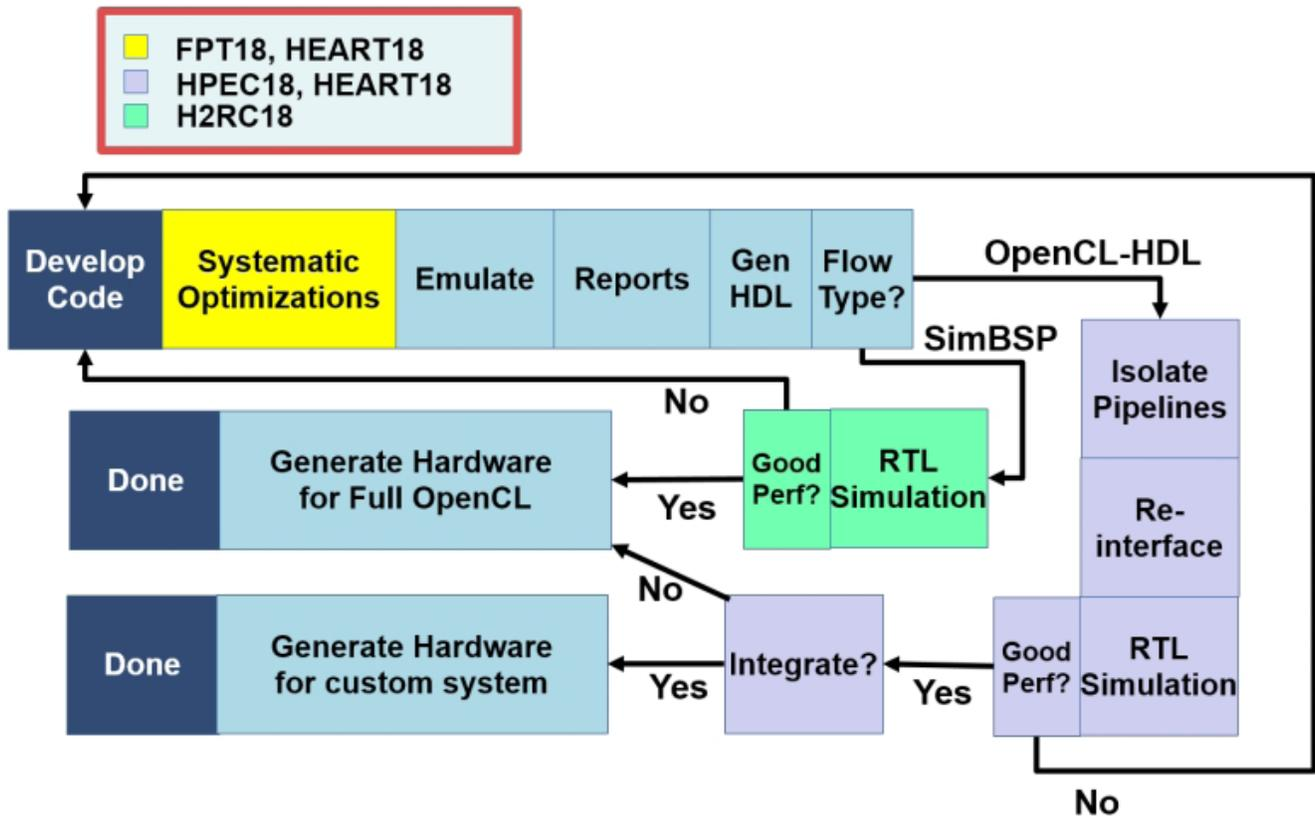
**1** The standard Intel® FPGA SDK for OpenCL™ technology toolflow is shown in light blue. Our augmentations to the standard toolflow are shown in yellow, green, and purple. This article describes the systematic optimizations.
